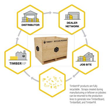
they will be cleaned, refined, and turned into wood fiber insulation. These recycled scraps are considered certified sustainable under the FSC Chain of Custody rules.
