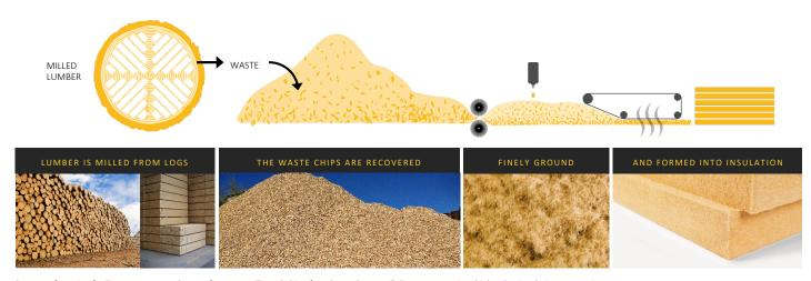
Our manufacturing facility converts wood waste from sawmills and chips from low-value, small-diameter trees into high-value insulating composites
